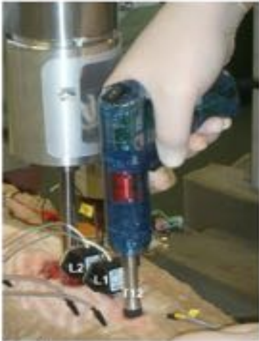
Figure 1 Experimental setup illustrating the Impulse Adjusting Instrument ® positioned over the T12 spinous process and the two tri-axial accelerometers rigidly attached to stainless steel pins at L1 and L2.
